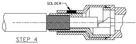
SEAT FERRULE ON BODY AND SOLDER FERRULE TO BODY THROUGH SOLDER HOLE. CLEAN.
