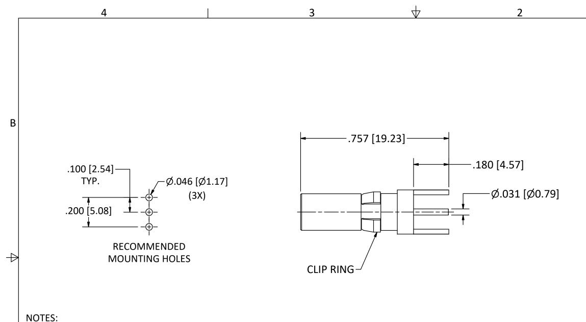
1. SPECIFICATIONS PER IDS-26. HOUSING: D-SUBMINIATURE, SIZE 8 CAVITY.
