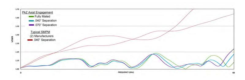
The PkZ provides a constant impedance profile over wide gaps in the mating interface thus, minimizing negative impact on VSWR.
