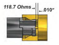
Impedance changes in a standard SMPM coaxial connector interface as a gap is introduced due to expected mating tolerances.
