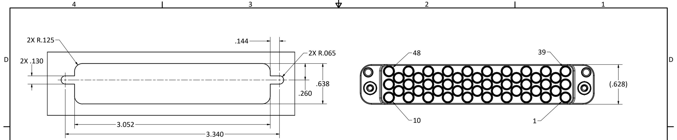
**RECOMMENDED PANEL MOUNTING CUT OUT (MAX. THICKNESS .125)**
